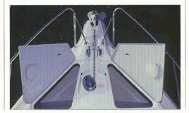
attention to detail. Two rope lockers compliment the electric anchor winch system; the unique Whittley standthrough sun roof (ideal when trying to choose the best track into a coral lagoon); the rigid hardtop over the cockpit for weatherproofing and vitally needed shade control; the standard solar panel and battery management system . . . this is truly a 'one of a kind' *Australian* cruiser reflecting decades of experience on Australian waters. The rear cockpit of the Cruisemaster 700
