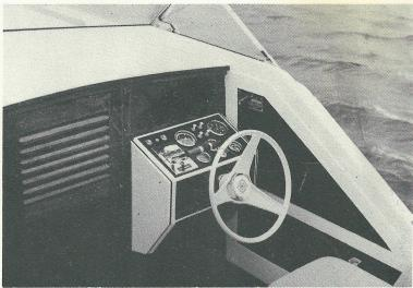
Cabin interior is fully lined with carpet and has a recessed vinyl ceiling. There is adequate sound-proofing insulation under the ceiling and on the decks.
